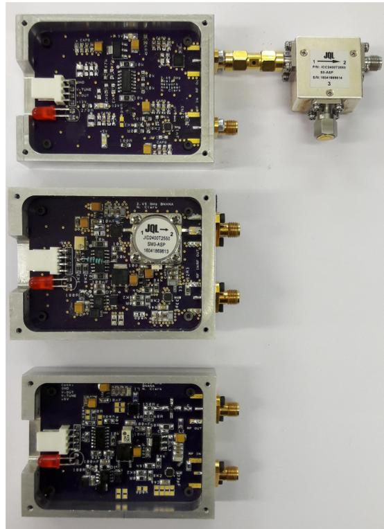
FIGURE 6.2: Photograph of BSA prototype circuits. From the top referred to as A, B and C. Prototype A pictured with connectorised circulator attached.
