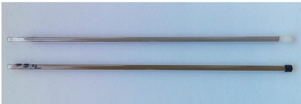
FIGURE 3.25: Ti6Al4V colour change after heat treatment under a small butane torch.
