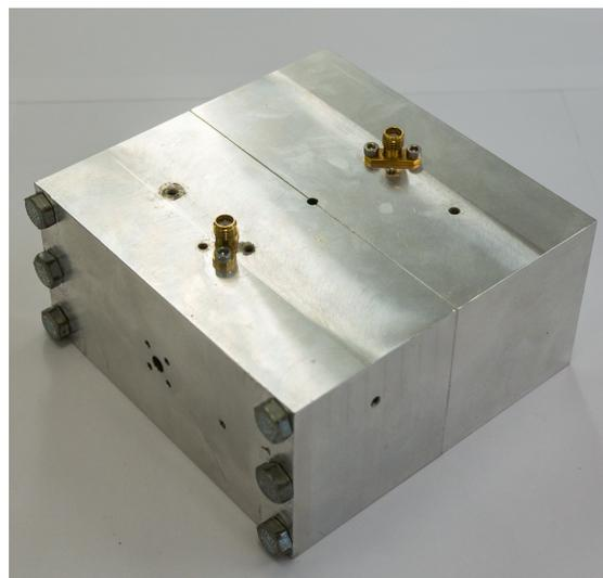
FIGURE 3.30: Aluminium  $TM_{010}$  measurement cavity used for electric field measurements.
