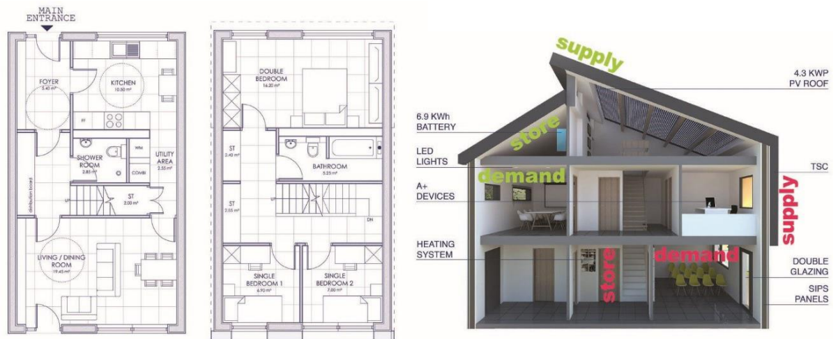
Figure 2-42: Plans and a 3d section showing demand, supply and storage locations (LCRI 2015)
