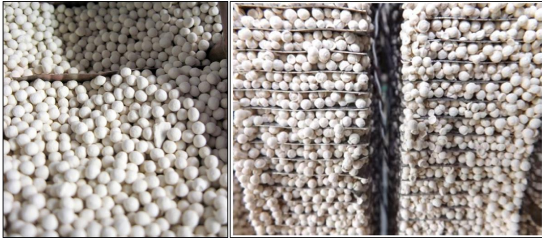
Figure 3-16: (left) Loose zeolite pellets (Fraunhofer 2012); (right) closed sorption system zeolite (De Boer et al. 2014)
