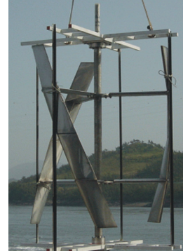
Figure 1.7: VATT prototype from Han et al. [2013] tested in their stage I phase.
