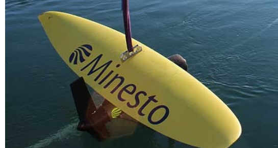
Figure 1.9: Tidal kite prototype developed by Minesto Ltd. Source: Minesto Limited .
