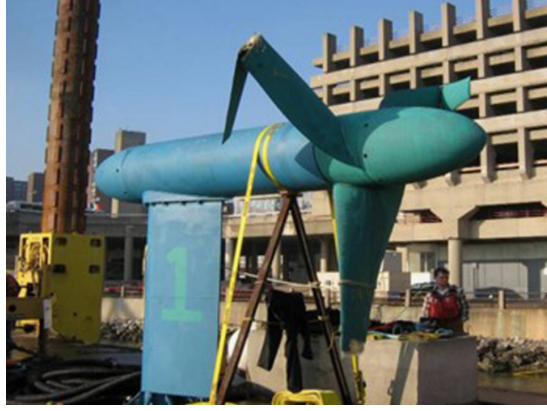
Figure 1.12: Verdant tidal current turbine after a structural failure in a blade. Source: Li et al. [2016b]
