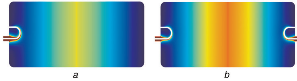
Fig. 4 Electric field distribution in cavity resonator with water sample at 25°C in case of
