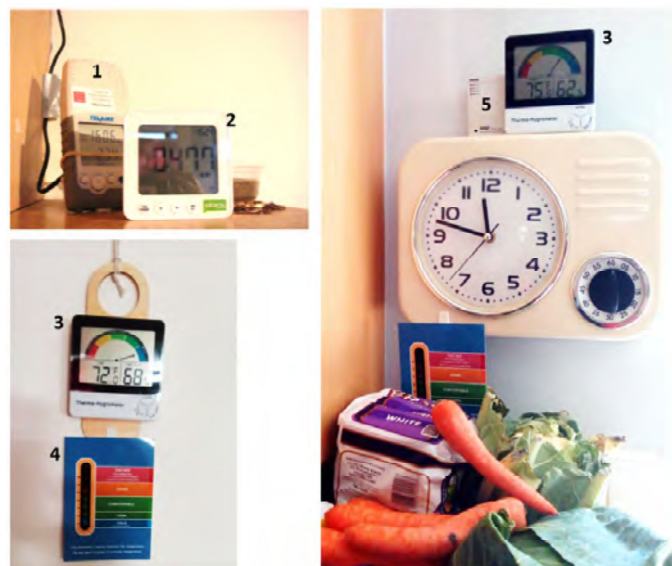
Figure 2 View of the monitoring equipment after installation. (1) CO 2 monitoring, (2) electricity meter, (3) therma-hygrometer, (4) temperature gauge and (5) HOBO datalogger.
