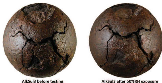
Figure 9. Physical condition of alkaline sulfite treated cannon ball before oxygen consumption testing (left) and after test runs through from 20% RH to 50% RH (right) (diameter 100mm)
