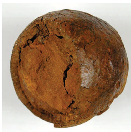
Figure 2. Cast iron cannon ball showing break up at metal/corrosion layer interface (diameter 65mm)
