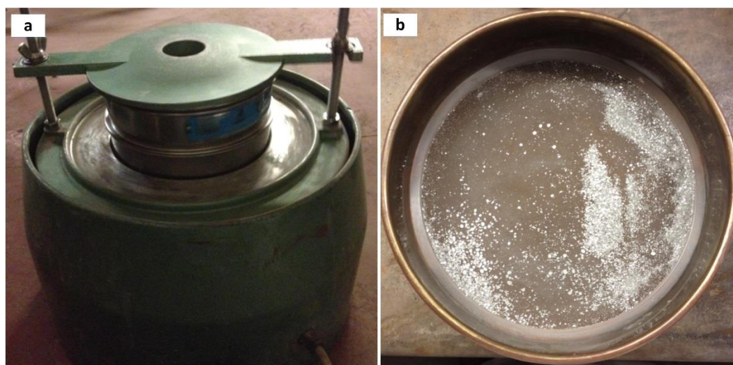
Figure A-3: The employed shaker and produced flake-like powders.
