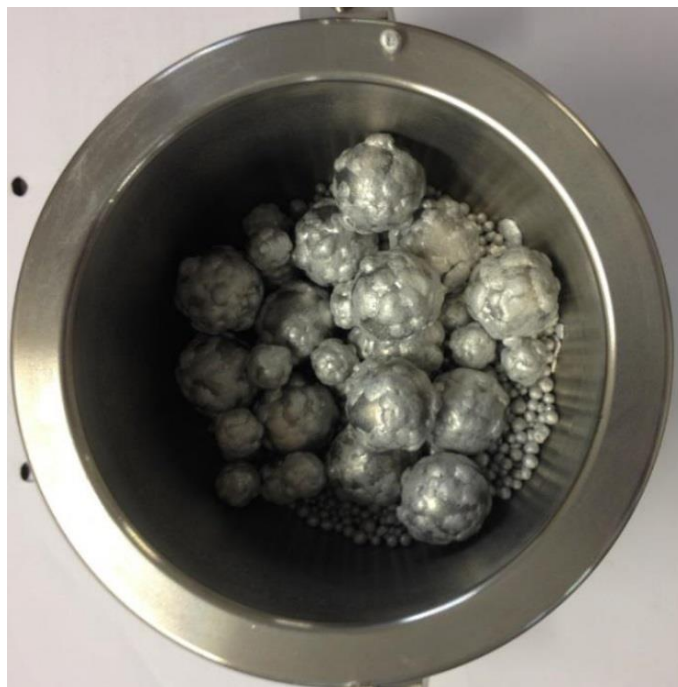
Figure A-2: Ball-milled pure Al for 6 hours without PCA.
