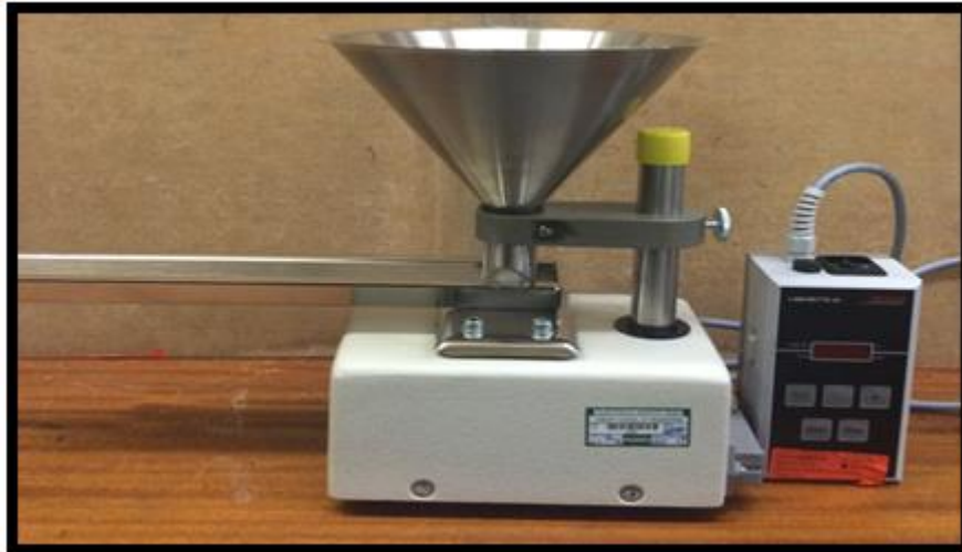
Figure 5-3 The fuel feeder (Fritch vibrating feeder).
