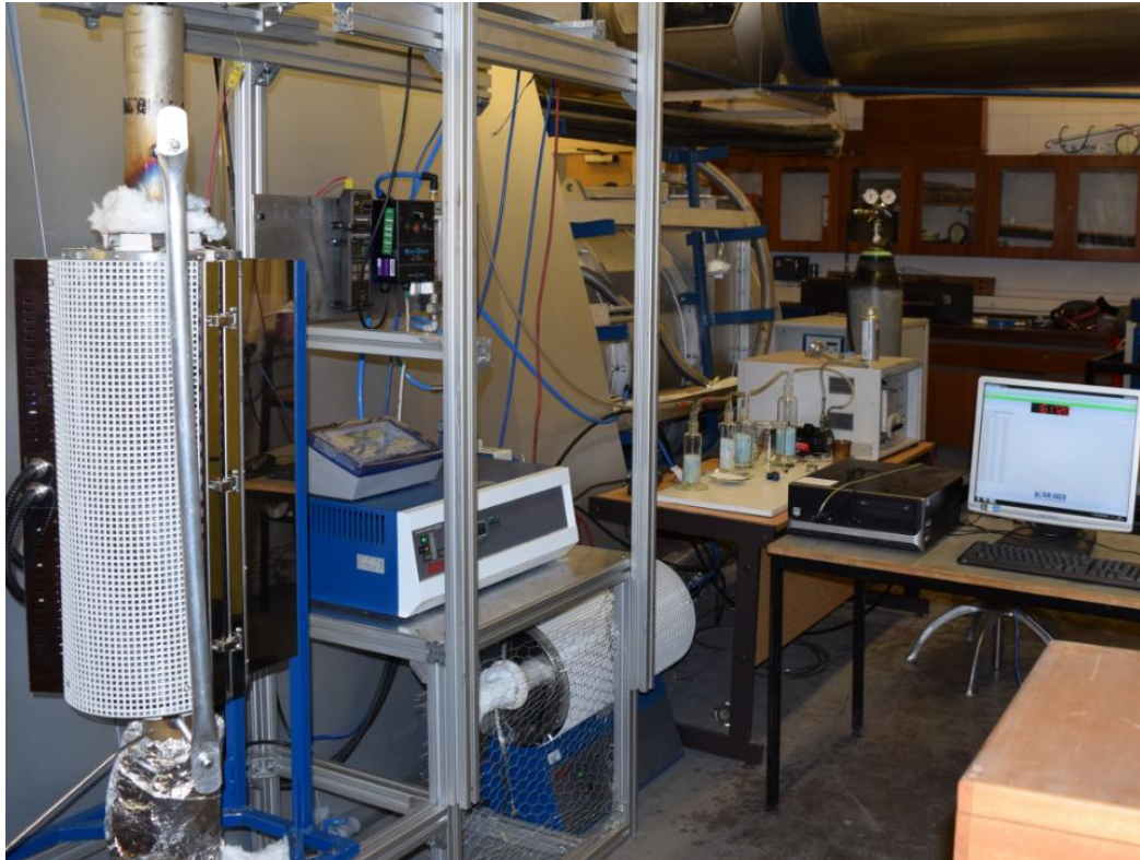
Figure 5-2. Thermogravimetric fluidised bed gasifier.
