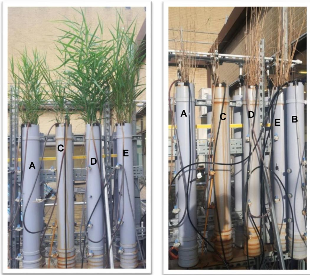
**Figure 5. 1** Constructed wetland system showing: (1) first period of operation on the left, and (2) second period of operation on the right.
