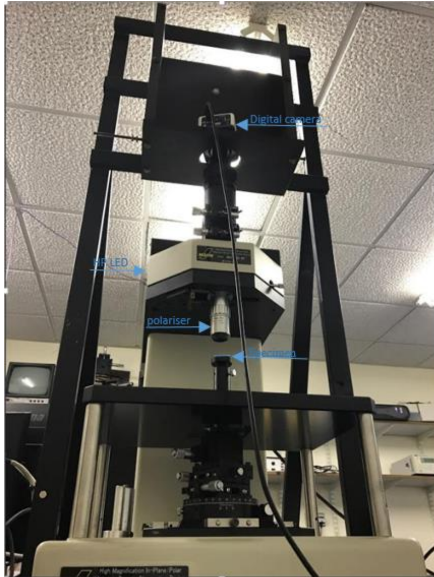
Fig 8-15 High magnification in-plane/polar magnetic domain observation device.
