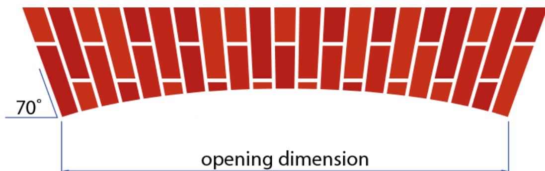
Figure 3.5: Semi-raised flat gauge arch (Prefabricated Arches, 2017)
