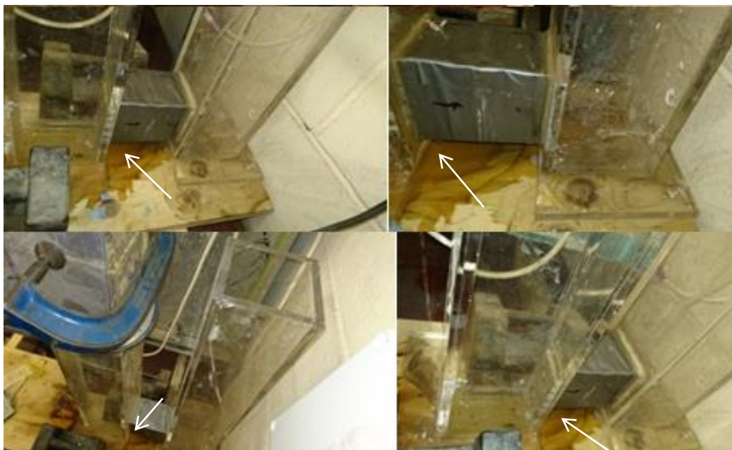
Figure 5.17 – Leaking tanks (not to scale, leaks shown with arrows)
