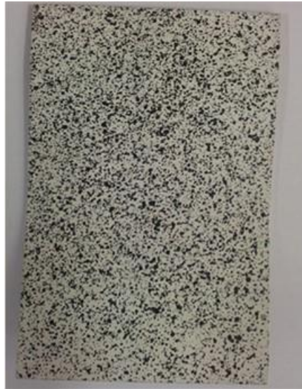
Figure 3.23: Speckle pattern of the pristine specimen used in buckling tests (Chapter 4).
