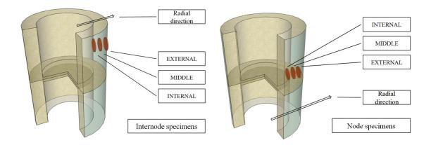
Figure 6.2.2 The cutting position of bamboo specimens in the radial direction
