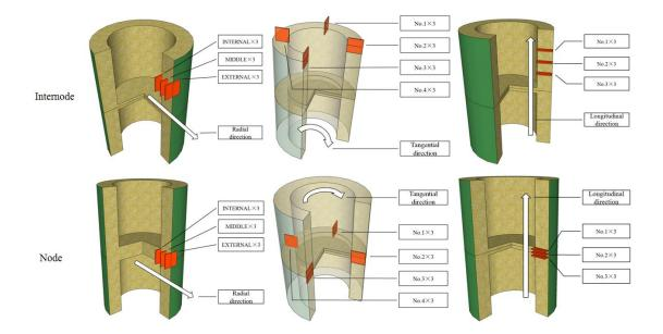
Figure 5.2.2 The cutting position of Moso bamboo specimens
