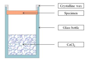
Figure 6.2.5 Assemblies for water vapour diffusion resistance factor measurement
