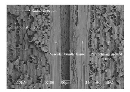
Figures 6.3.4 A BSE image of a bamboo radial-longitudinal section (×100)
