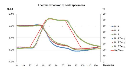
Figure 8.3.4 The thermal expansion of node specimens in the tangential direction
