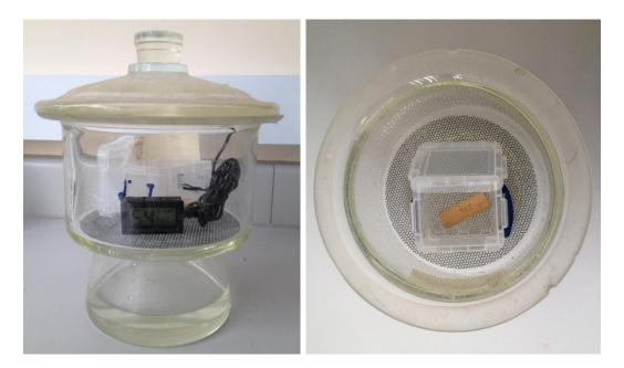
Figure 7.1.6 The desiccator assembly
