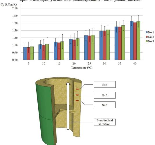
Specific heat capacity of internode bamboo specimens in the longitudinal direction
