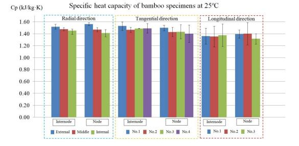
Figure 4.3.7 Average specific heat capacity comparison at 25 °C.
