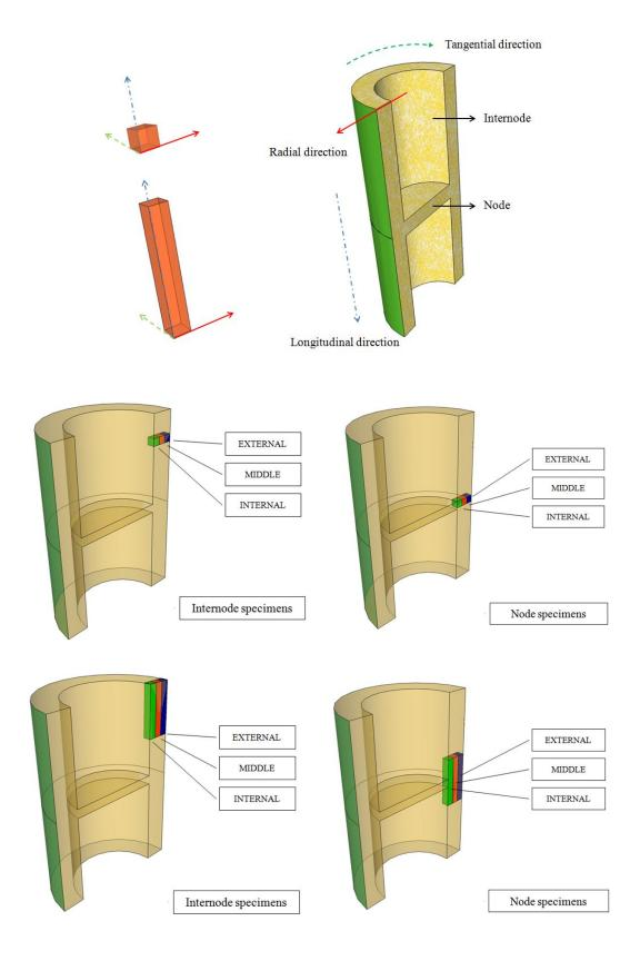
Figure 8.2.1 Cutting position and directions of bamboo specimens
