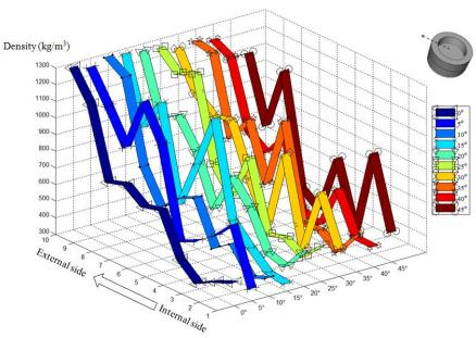
Density distribution in the radial direction of internode specimen
