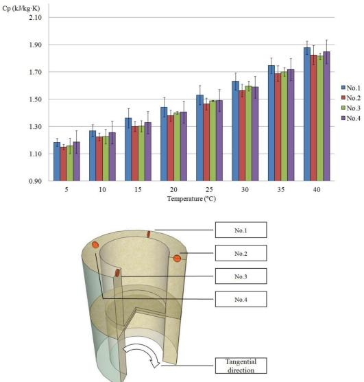
Specific heat capacity of internode bamboo specimens in the tangential direction
