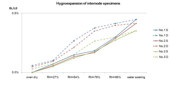
Figure 8.3.11 The hygroexpansion of internode specimens in the longitudinal direction
