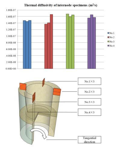
Figure 5.3.3 Thermal diffusivity of node bamboo specimens in the tangential direction
