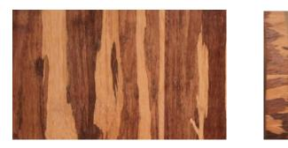
Figure 1.2 (a): Recombination bamboo panel front view (b): section view
