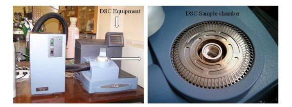
Figure 2.2 Differential scanning calorimeter (DSC)
