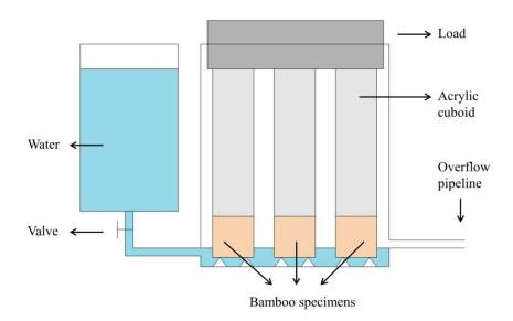
Figure 7.2.2 Testing apparatus for water adsorption coefficient measurement
