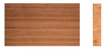
Figure 1.3 (a): Laminated bamboo panel front view (b): section view
