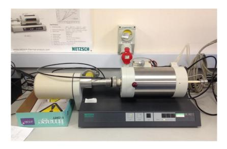
Figure 2.8 Dilatometer for thermal expansion measurement
