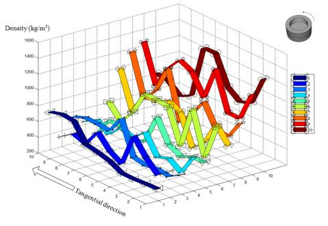
Density distribution in the tangential direction of node specimen
