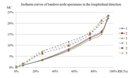
Figure 7.1.9 Sorption isotherm curves in the longitudinal direction
