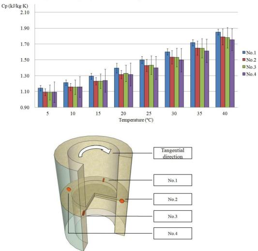
Specific heat capacity of node bamboo specimens in the tangential direction
