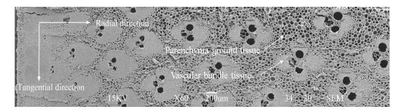
Figure 6.3.2 The SEM image of a bamboo specimen (×60)
