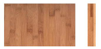
Figure 1.6 (a): Laminated bamboo panel front view (b): section view
