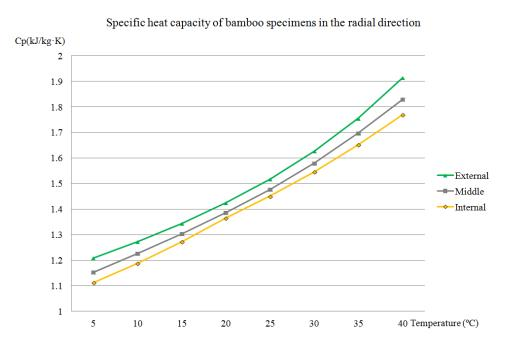
Figure 9.2.6 The average specific heat capacity results of bamboo specimens
