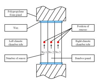
Figure 9.2.3 The edge section of bamboo panels with the temperature and RH sensors
