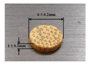
Figure 4.2.1 The dimension of the bamboo specimen
