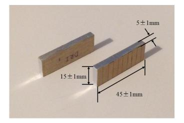
Figure 7.1.5 The size of specimens
