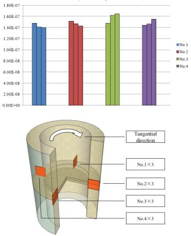
Thermal diffusivity of node specimens (m<sup>2</sup>/s)
