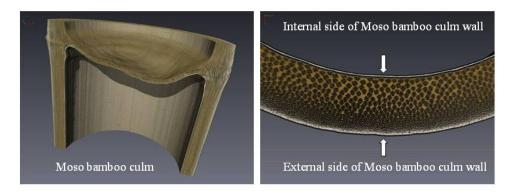
Figure 2.1 The non-homogenous section view of Moso bamboo
