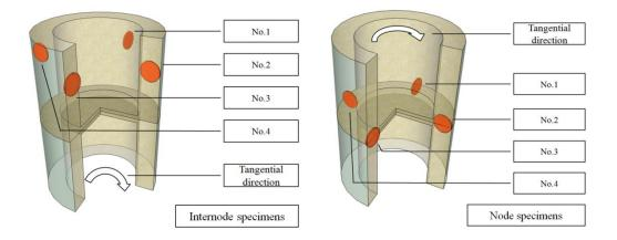
Figure 6.2.3 The cutting position of bamboo specimens in the tangential direction
