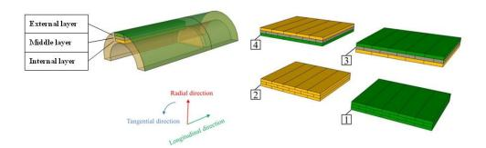
Figure 9.2.1 Four types of bamboo laminated panels
