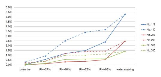
Figure 8.3.8 The hygroexpansion of node specimens in the radial direction
