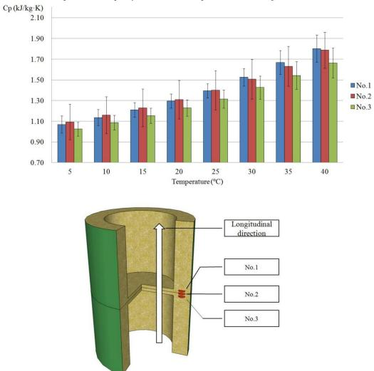
Specific heat capacity of node bamboo specimens in the longitudinal direction
