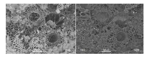
Figure 3.3.3 Comparison between the BSE image and secondary electron (SEM) image
