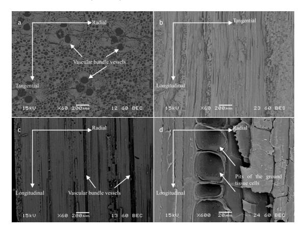
Figure 4.3.8 (a) The radial-tangential section view of the Moso bamboo BSE image. (b) The tangential-longitudinal section view of the Moso bamboo BSE image. (c) The radial - longitudinal section view of the Moso bamboo BSE image. (d) The radial -longitudinal section view of the Moso bamboo BSE image at a high magnification.
