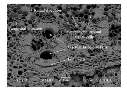
Figure 6.3.3 A BSE image of a bamboo cross-section (×100)
