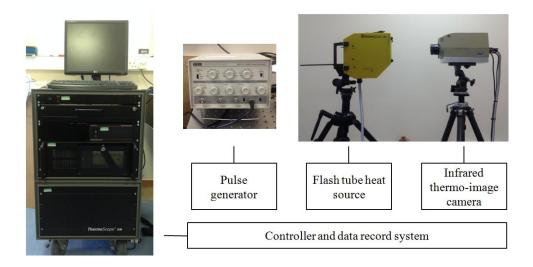
Figure 5.2.3 Flash tube system for thermal diffusivity measurement
