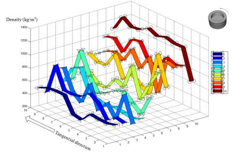
Density distribution in the tangential direction of internode specimen
