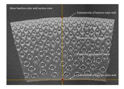
Figure 9.1.1 Section view of a Moso bamboo culm wall
