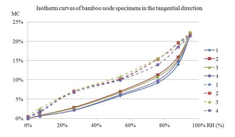
Figure 7.1.8 Sorption isotherm curves in the tangential direction
