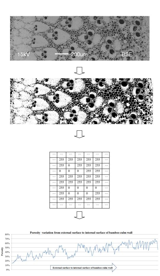
Figure 3.3.4 The transfer procedure from BSE image to porosity values
