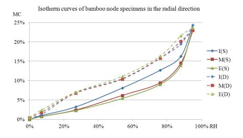
Figure 7.1.7 Sorption isotherm curves in the radial direction
