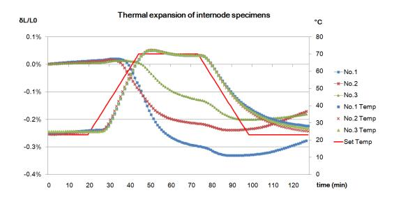
Figure 8.3.3 The thermal expansion of internode specimens in the tangential direction
