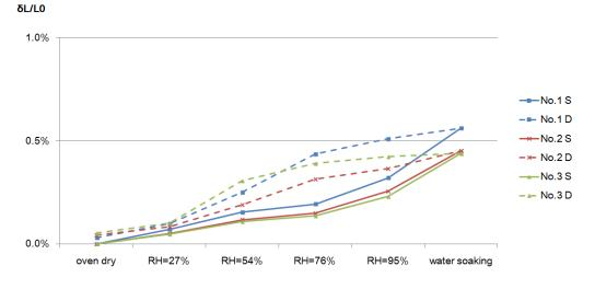
Figure 8.3.12 The hygroexpansion of node specimens in the longitudinal direction
