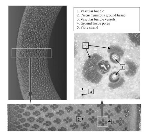
Figure 3.1.2 Anatomical features of Moso bamboo in the radial direction (Huang et al. 2014)
