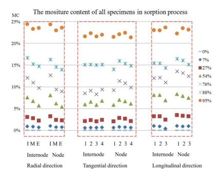
Figure 7.1.10 The moisture content of all specimens in sorption process
