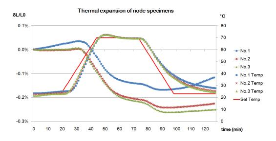
Figure 8.3.2 The thermal expansion of node specimens in the radial direction
