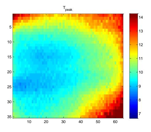
Figure 2.3 Peak temperature test image of the specimen in flash tube experiment
