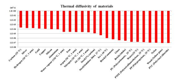
Figure 5.3.7 Thermal diffusivity of materials
