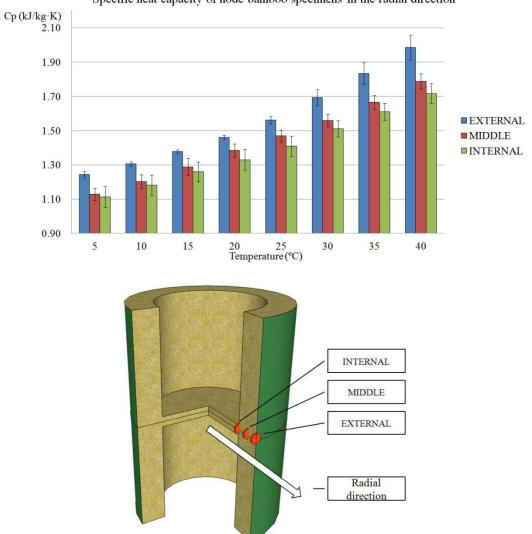
Specific heat capacity of node bamboo specimens in the radial direction
