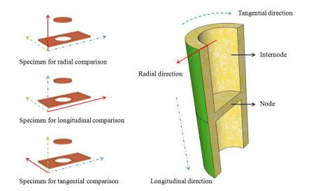
Figure 4.2.2 Nomenclature of the directions of specific heat capacity measurements
