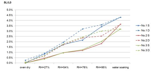
Figure 8.3.10 The hygroexpansion of node specimens in the tangential direction
