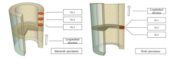
Figure 6.2.4 The cutting position of bamboo specimens in the longitudinal direction
