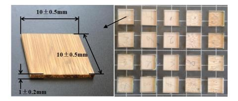
Figure 5.2.1 The dimension and fixation of Moso specimens
