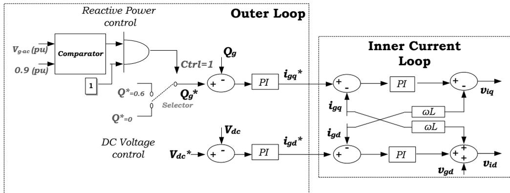
Figure 5- 5: A supplementary control in unity power factor control mode
