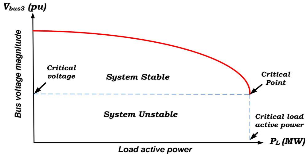
Figure 3- 2: Typical P-V Curve
