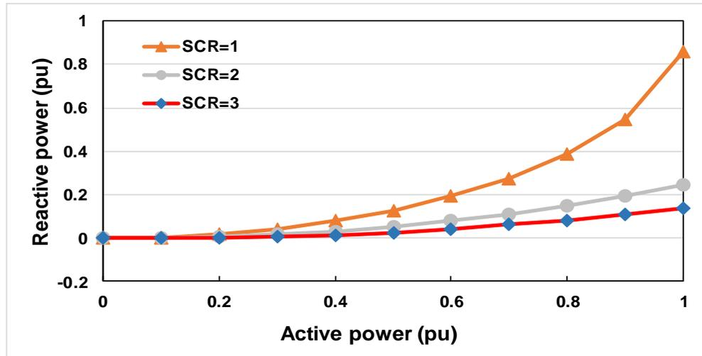
Figure 4- 3: The PQ curve for different SCR values
