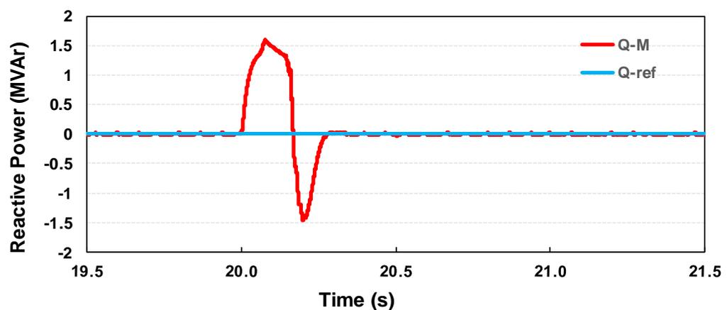
(d) Reference &amp; measured reactive power of grid side converter
