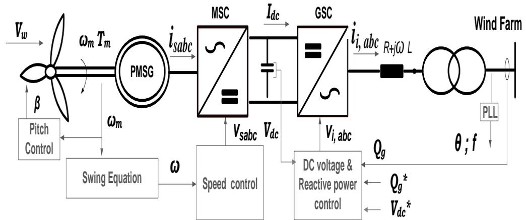
Figure 5- 2: Wind Farm Diagram
