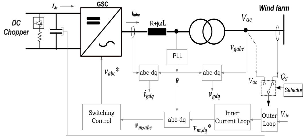
Figure 5- 4: Grid side converter structure
