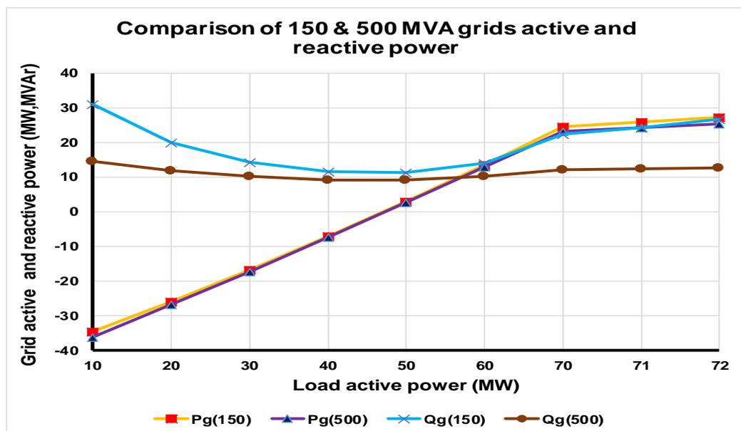
Figure A- 1: Comparison of 150 and 500 MVA grid active and reactive power
