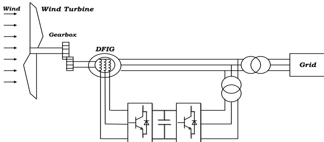
Figure 1- 3: Variable-speed wind turbine with a DFSG
