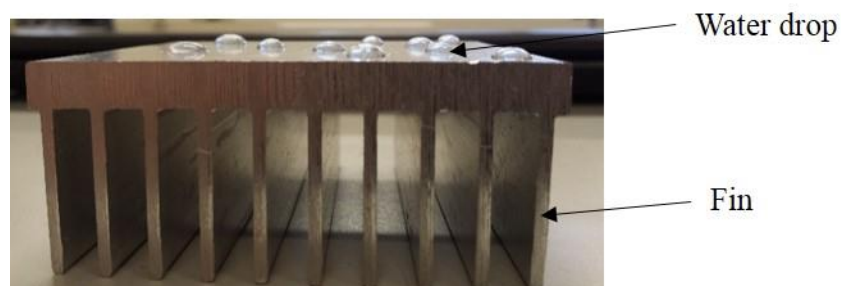
Figure 3.24: A photograph of water drops on the surface of aluminium condenser.
