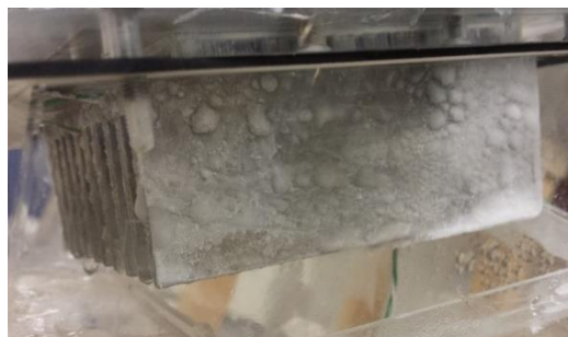
Figure 6.9: A photograph of ice formation on the condenser during an operation, in which the temperature of the sample water is 30^{\circ}\text{C} and the Peltier current is 10 A.
