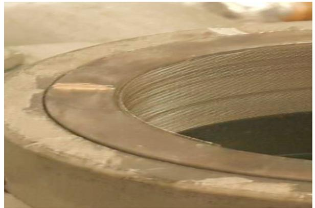
Figure 3. Nozzle with 150µm wire mesh.
