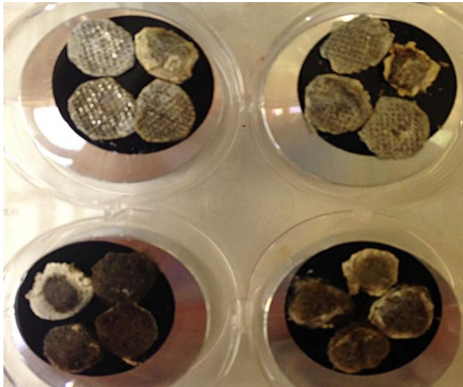
Figure 3.6: Meat and dressings processed in-situ for SEM
