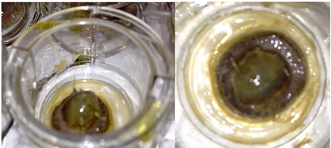
Figure 3.3: A meat model with NSHD after 24 hours of growth Meat with dressing in an insert within a well of a clean plate, with remnants of TSB culture
