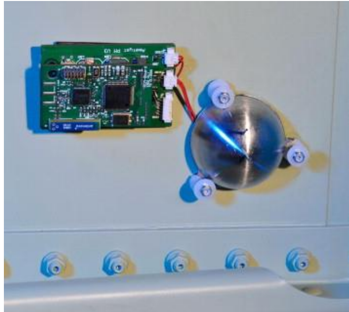
Figure 2.15 Prototype of ASHM sensor powered by thermal energy harvester attached to the inside of an aircraft hull (Samson, Kluge et al. 2011)
