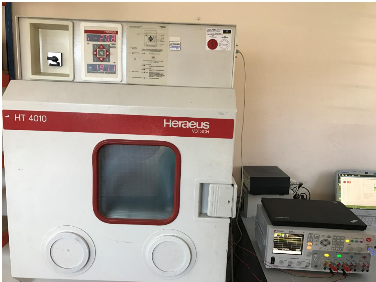
Figure 3. 12 Climatic chamber set up for LTC3109 V_{out} and V_{store} measurement and tested on a temperature range of -40^{\circ}\text{C} to +40^{\circ}\text{C}
