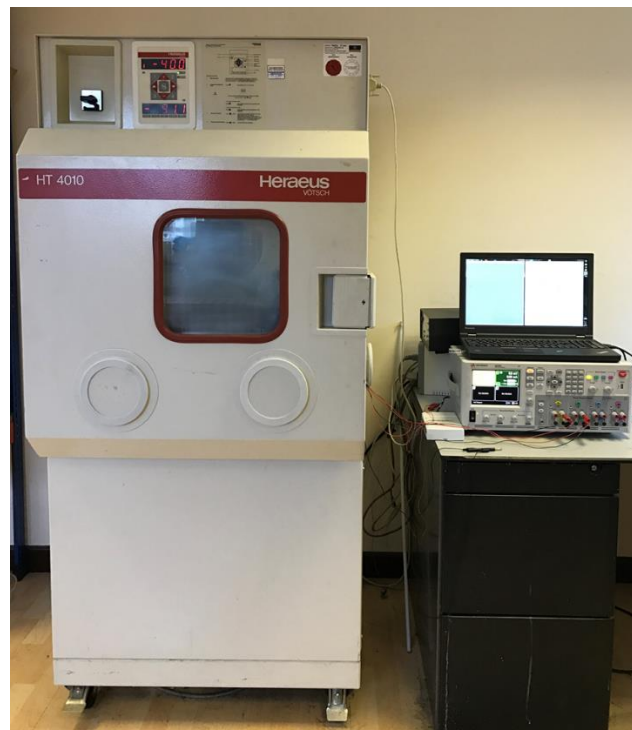
Figure 4.10 Experimental set up for characterisation of energy storage elements under the different temperature range with climatic chamber
