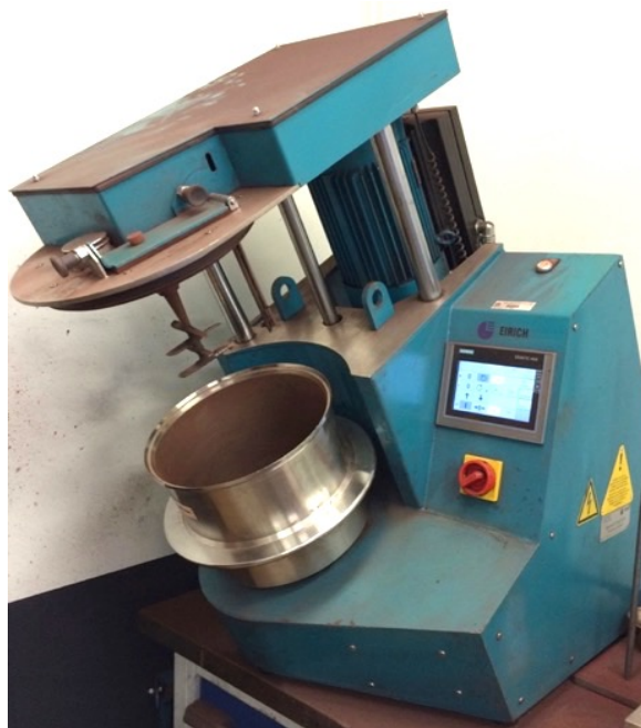
Figure 3.10 – Eirich mixer (TATA Steel Europe RD&T)
