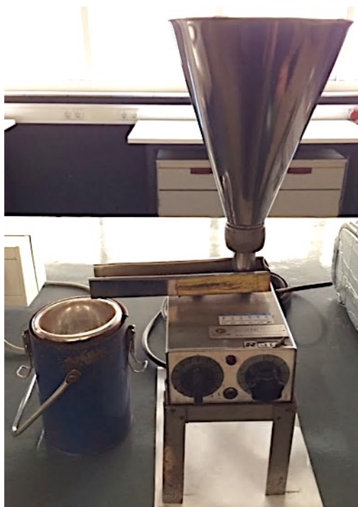
Figure 3.13 – Vibrating feeder and liquid nitrogen pot
