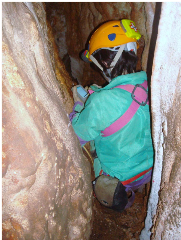
Fig. 7. P. Filippatou mapping in Charambos tou Giorgi pothole, with DistoX1 and PDA during the Kythera Speleological Project. (courtesy of the author)
