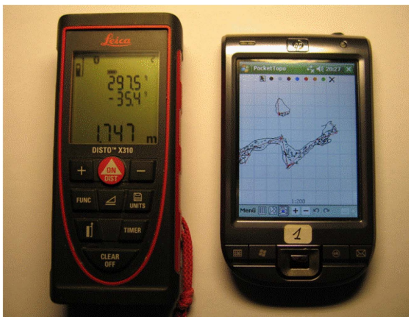
Fig. 2. Leica DistoX2 and PDA with PocketTopo software.
