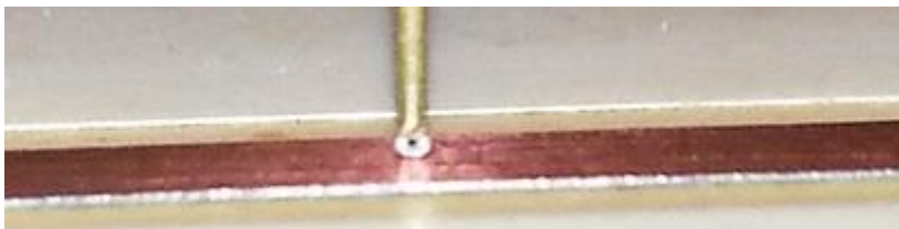
Figure 5-31 The plane containing the loop is parallel to the length of the microstrip line.
