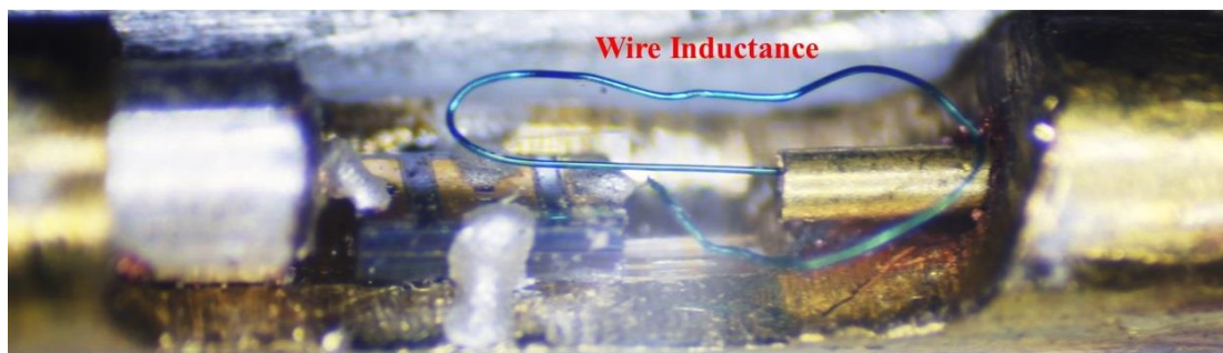
Figure 4-22 The wire inductance created by extending the central conductor of the short input coaxial cable ( L = 6 mm) inside the housing of the voltage probe.
