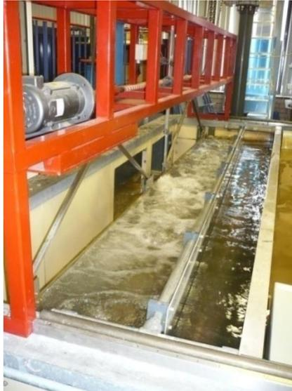
**Fig. 4.5** The tide-generating weir
