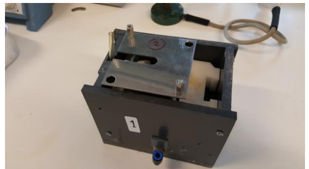
g) The main box, shear box and luck plate
