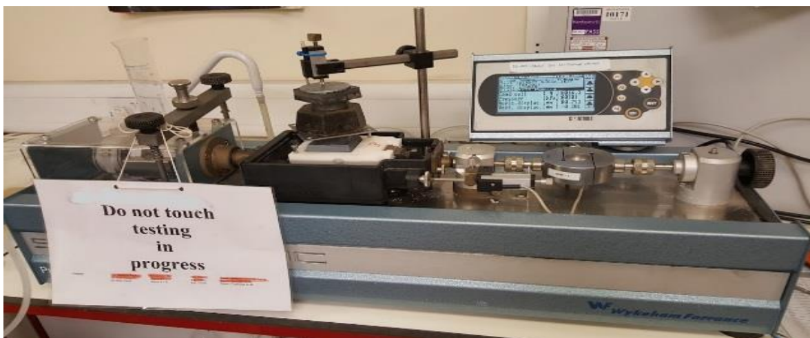
l) Direct shear equipment using weight blocks
