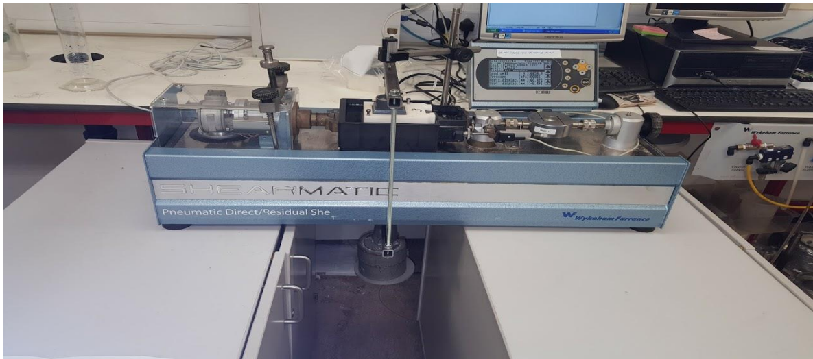
m) Direct shear equipment using loading frame
