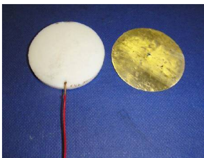
Figure 2.13: First-generation reactor electrode-wire connection.
