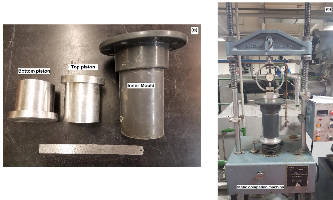
Fig. (3.22): (a) Specimen mould and pistons used during preparation of compacted specimens and (b) Static compaction setup
