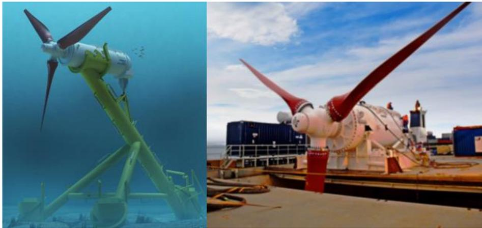
Figure 2.16 Structure of the HS1000 tidal turbine system Source: McEwenet.al.2012
