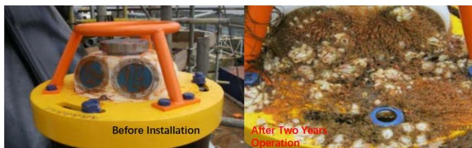
Figure 2.27 Changes of seabed-based ADCP after two years of operation. Source:
