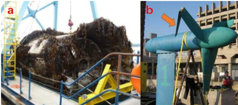
Figure 2.34 Examples of the faulty tidal turbine system. Sources: Elasha et al, 2014 and Zhou et al, 2016.
