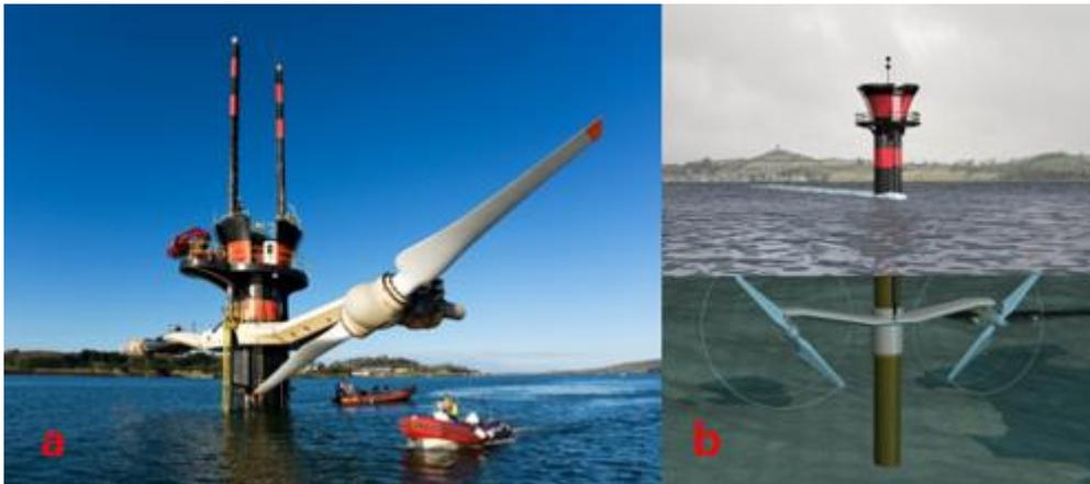
Figure 2.11 Seagen S tidal turbine located in Strangford Lough; a) shows that rotor blades are lifted for inspection; Right) shows illustration of Seagen S system in operation. Source: MCT, 2008
