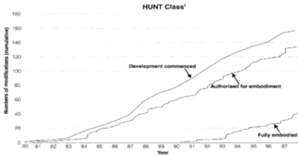
Figure 2.1: Modification volumes to the Hunt Class Minesweeper (NAO 1998)
