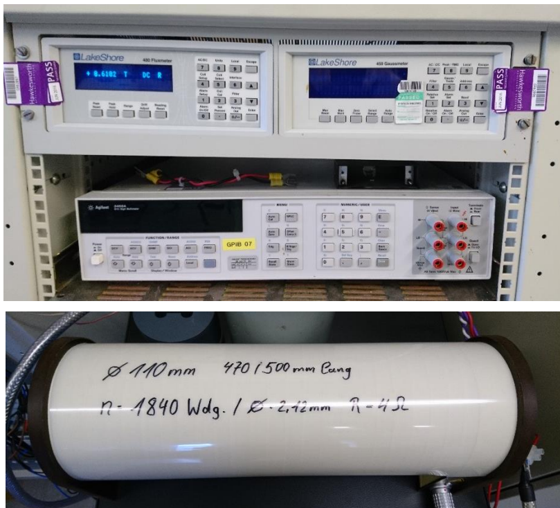
Figure 47: Top: Lakeshore Fluxmeter and Kepco power unit. Bottom: 1840 turn solenoid used for generation of the magnetic field for Hall probe calibration.
