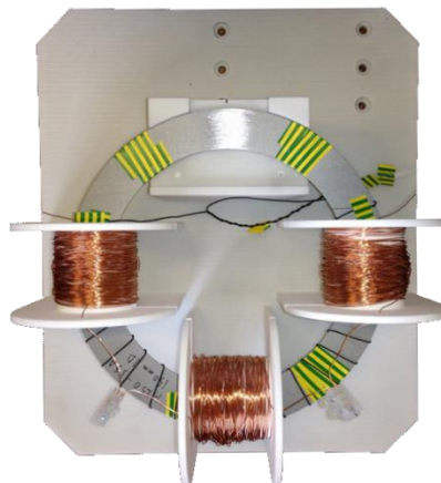
Figure 36: Coil system design consisting of three winding formers with a 150 mm ID ring sample
