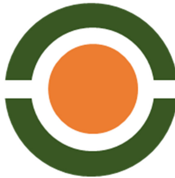
Figure 3.2 A schematic of the illumination beam (green annulus) and imaging beam (orange circle) as seen in the pupil plane. The illumination annulus has an outer diameter of 6.7mm, inner diameter of 4.7mm and the imaging beam has a diameter of 3.2mm.
