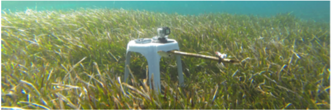
Figure 82. Final GoPro monoBRUV design used in this study. The GoPro was attached to a plastic frame and directed towards a bait box located at the end of a pole. The frame was weighted with two 1kg dive weights to ensure stability on the seafloor. This design enabled a snorkeler to deploy the system by hand in water depths of <10m.
