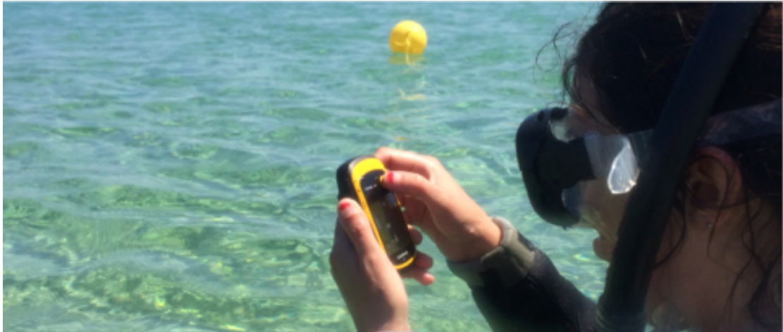
Figure 52. A Garmin eTrex 10 GPS unit was used to 'ground truth' study locations.
