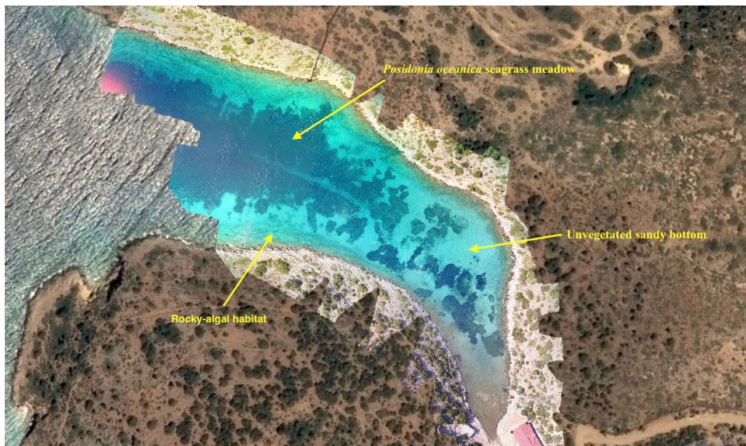
Figure 58. A Google Maps™ satellite baselayer in QGIS showing the successful export of a georeferenced orthomosaic layer derived from photographic images
