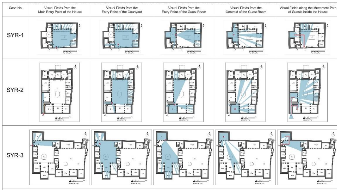
Figure 4.51: Samples of isovist analyses for three traditional courtyard houses located in Syria, produced by ‘Syntax2D 1.3.0.7’ software
