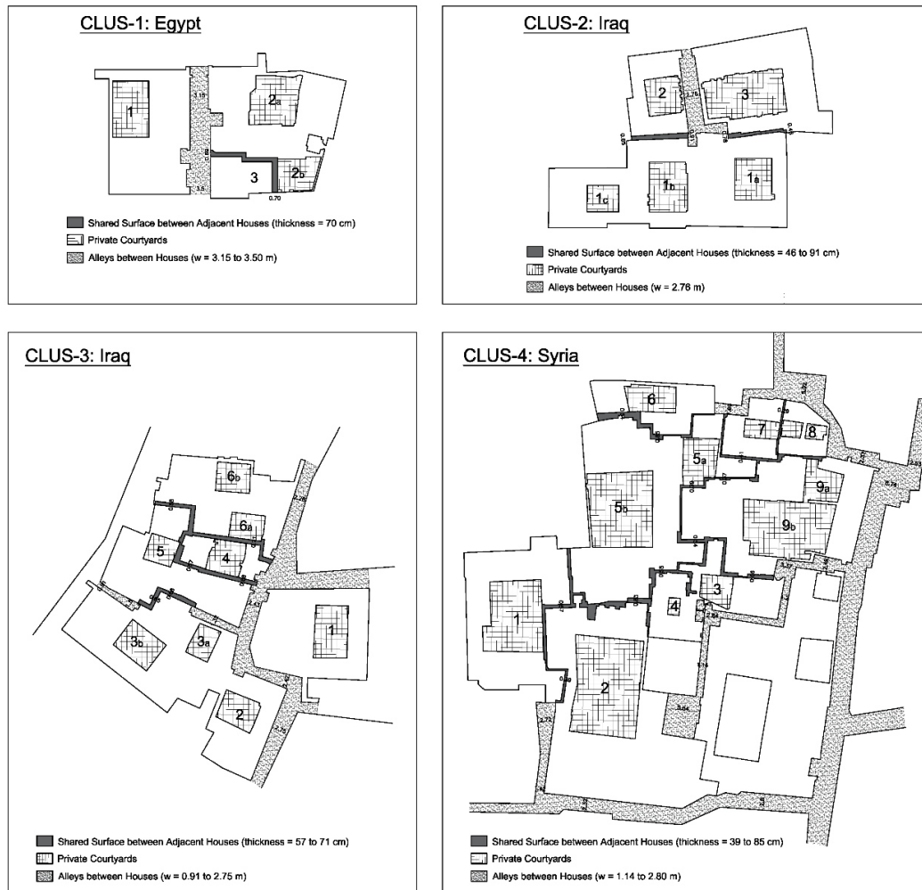
Figure 4.99: Shared walls and alleys between adjacent houses in traditional residential quarters
