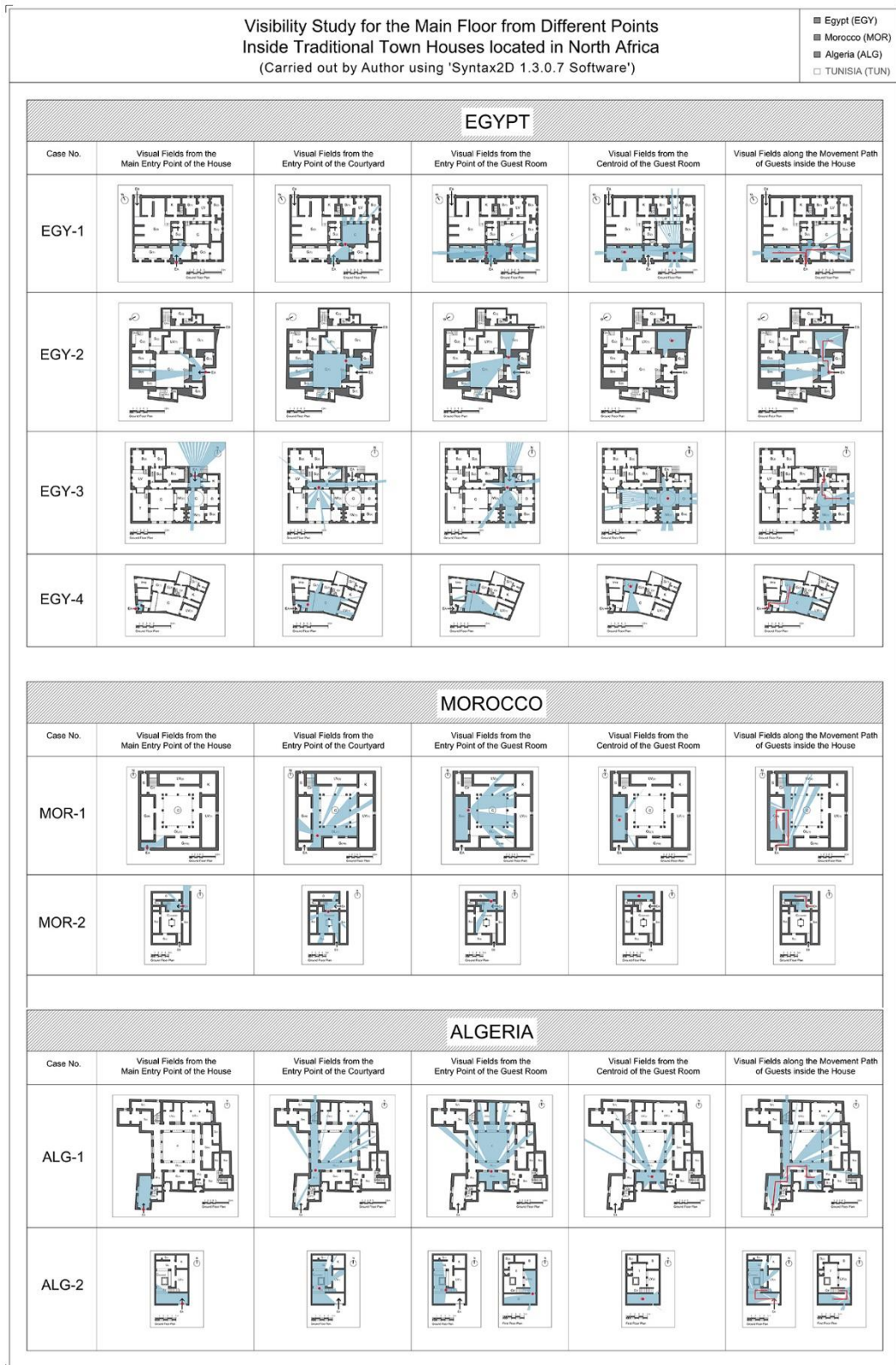
Figure 4.82: Isovist analysis for traditional courtyard houses located in North Africa, produced by 'Syntax2D 1.3.0.7' software
