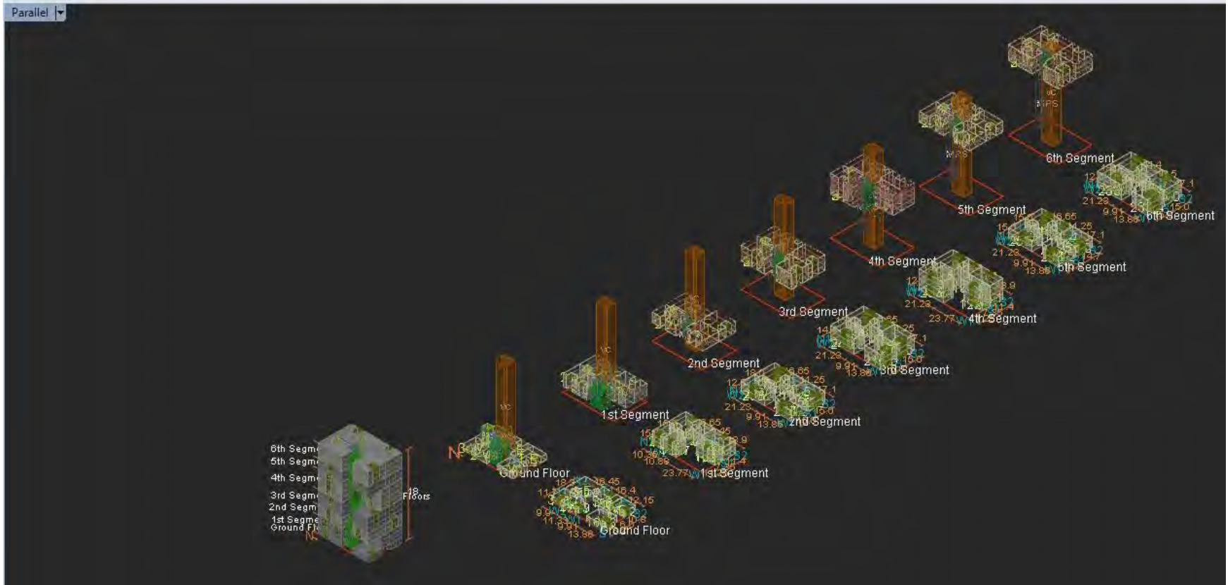
A screenshot showing the generated three-dimensional views for the building and for each segment carried out by the system
