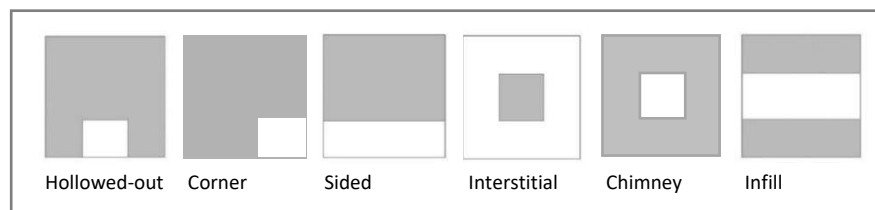
Figure 2-6. Spatial configuration of skycourts in high-rise office buildings (the white shaded zone represents the skycourt)
