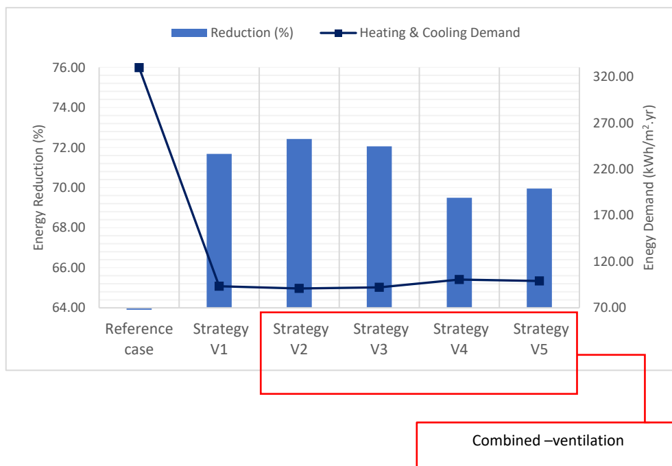
Figure 5-66. Annual total heating and cooling demand comparison in the sided skycourt (C) building: ventilation strategies
