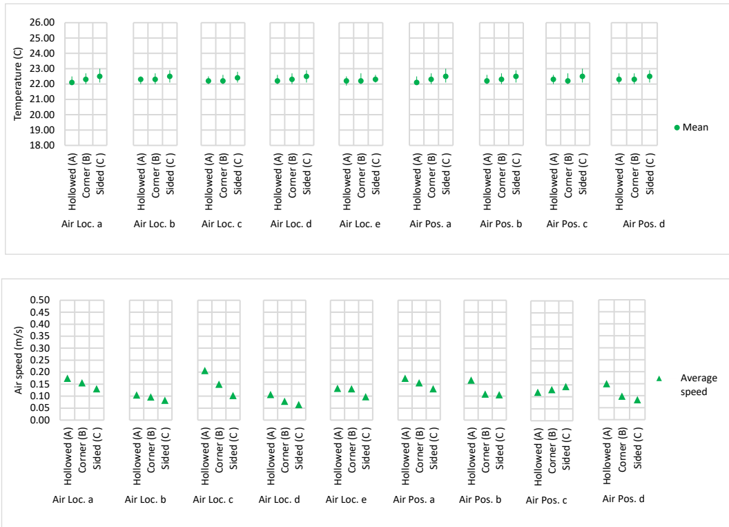
Figure D-18. Thermal conditions at the occupancy level of the (A) hollowed-out, (B) corner and (C) sided ventilated skycourts in mid-seasons cases: air inlet and outlet openings
