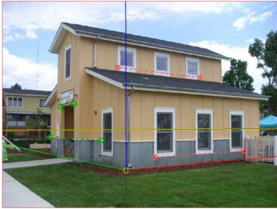
Figure 4 configuring the photos vanishing points using SketchUp.
