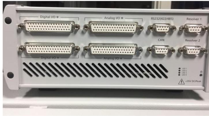
Fig. 5.9 The front panel of the dSPACE MicroLabBox
