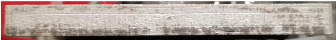
Figure 6-12. Image of the sample side painted with silver paint after three consecutive high current tests at 5, 6 and 7 kA peak.
