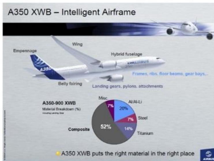
Figure 1-2. a) Boeing 787 Dreamliner made by 50% of composite materials. b) Airbus A350 XWB made by 52% of composite materials [3] [5].
