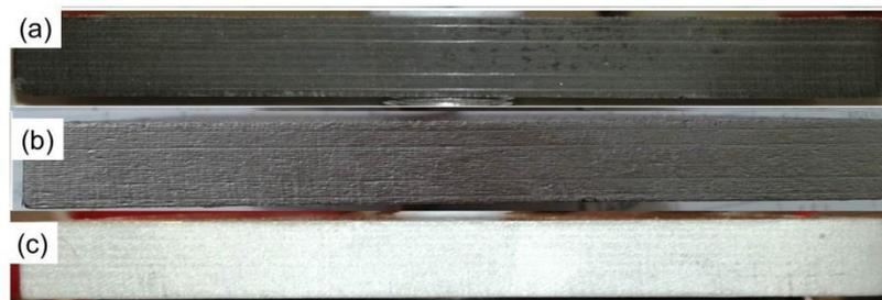
Figure 4-12. Contact sides of the samples: a) sample with no coating, b) sample with silver paint coating, c) sample with metal sputter coating.
