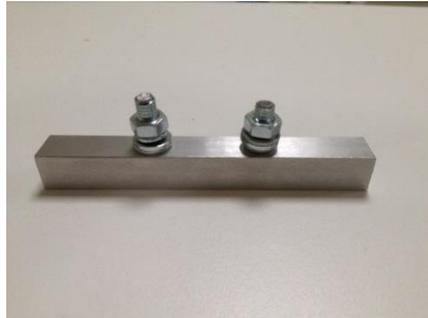
Figure 4-16. Aluminium electrode: the two screws and nuts are required to connect the electrode with the circuit through copper wires.
