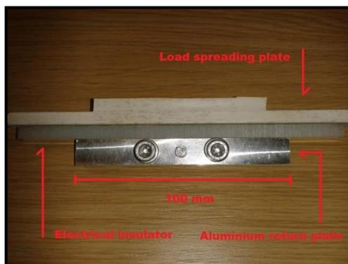
Figure 4-17. Load spreading plate with insulator and return metal plate.
