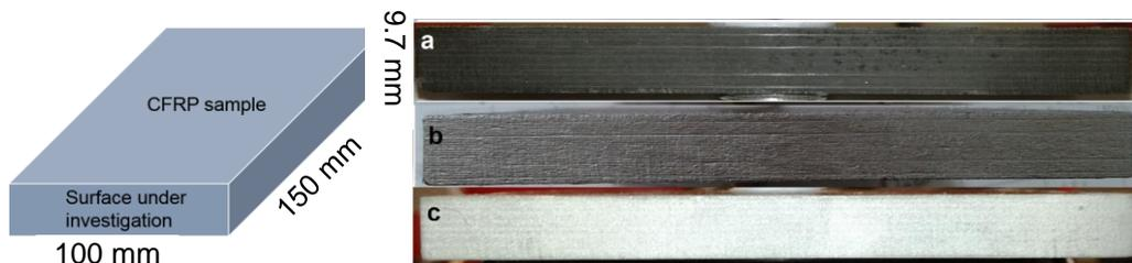
Figure 5-13. Surface of the sample under investigation: a) No-layer surface, b) silver paint surface, c) metal sputtering surface.
