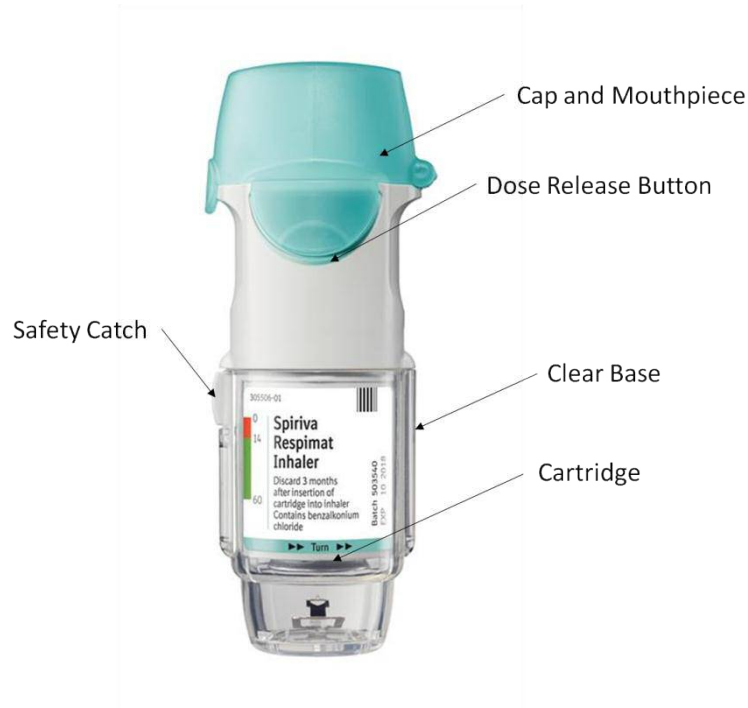
Figure 3. 2 Configurations of Respimat ® . During usage, the clear base is taken off and the cartridge is inserted into the inhaler. The clear base is put back with a half twist. Once the cap is opened the dose release button can be used deliver a dose.
