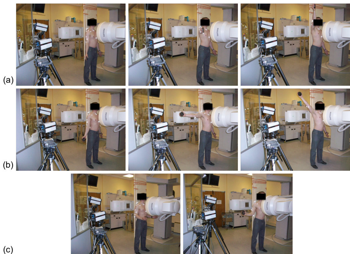
FIGURE 2.5: Simultaneous fluoroscopy and motion analysis recordings (a) frontal plane elevation, (b) scapular elevation and (c) external rotation
