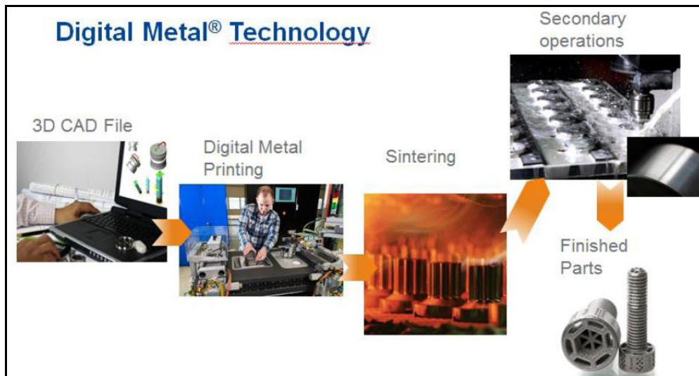
Fig. 2 Process diagram showing the Digital Metal® technology [43]
