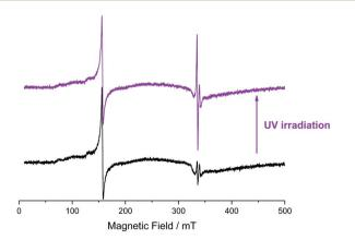
Fig. 4 Experimental X-band CW EPR spectra of the Fe–TiO $_2$  sample containing 0.07 at% of Fe, recorded at 120 K,  $1\times10^4$  receiver gain; 100 kHz modulation frequency; 5.0 Gauss modulation amplitude and 20.2 mW microwave power, before (black) and after (violet) *ex situ* UV irradiation at 77 K.
