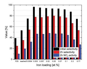
Fig. 6 The  $DeNO_x$ -performance of P25 samples grafted with different amounts of iron. Displayed are the initial nitrate selectivity (black) as well as the selectivity (red) and  $NO_x$  removal rates (green) after 2 h on stream.
