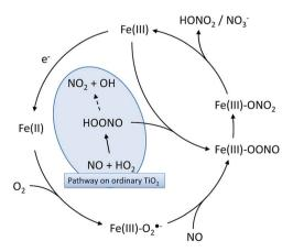
Fig. 11 The proposed reaction mechanisms for peroxynitrite/peroxynitrous acid isomerization on the grafted Fe(III) that would prevent NO<sub>2</sub> release through peroxynitrous acid decomposition.
