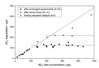
Fig. 8 The oxidation of  $NO_2$  over illuminated P25, grafted with 0.05 at% Fe, with varying inlet concentrations of  $NO_2$ . Shown are a freshly prepared sample (blue triangles) as well as ones which were already subjected to short (red filled circles) and long  $DeNO_x$  testing (black squares) procedures. Conditions according to ISO 22197-1, except inlet concentration.
