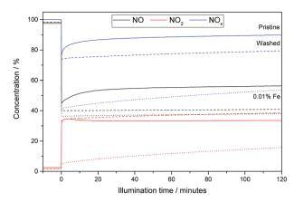
Fig. 5 The relative changes in NO (black),  $NO_2$  (red) and total  $NO_x$ -levels (blue) during a run of the ISO test 22197-1 with 1 ppm inlet concentration of NO. Represented are runs for pristine P25 (solid lines), washed P25 (slashed lines) and P25 grafted with 0.007 at% of Fe (dotted lines).
