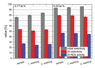
Fig. 9 Long-term stability and recycling tests of the modified photocatalysts. Shown is the  $DeNO_x$ -performance in terms of initial nitrate selectivity (grey) as well as the selectivity (red) and  $NO_x$  removal rates (blue) after 2 h on stream for a sample with 0.77 at% iron (left) and a sample with 0.05 at% iron (right) in 3 repeated cycles with washing steps in between.
