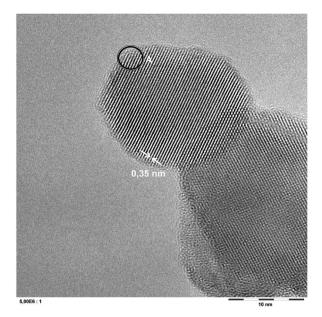
Fig. 1 A representative ATEM micrograph of a P25 sample grafted with 0.007 at% iron. The displayed lattice spacing of 0.35 nm corresponds to anatase  $\text{TiO}_2$ . The indicated area A was subjected to EDX analysis, *cf.* Fig. 2.
