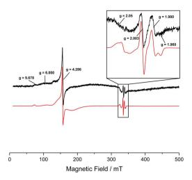
Fig. 3 Experimental (black) and simulated (red) X-band CW EPR spectra of the Fe-TiO<sub>2</sub> sample containing 0.07 at% of Fe, recorded at 120 K,  $1\times10^4$  receiver gain; 100 kHz modulation frequency; 5.0 Gauss modulation amplitude and 20.2 mW microwave power, prior UV irradiation. The region of the spectrum around free spin (i.e.  $g_e=2.0023$ ) is also shown enlarged.
