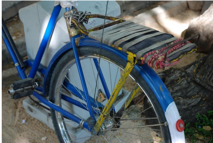
Figure 5.14 Heavy duty welded steel carrying rack on a respondent's Challenger, Rundu
