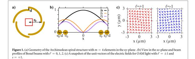
the vortex can be used to excite unusual transitions [30]. We analyse the response of a micrometer-sized Archimedean spiral structure to the excitation with OAM light, showing that the topological charge of the vortex can be controlled by exciting with light having different OAM.
