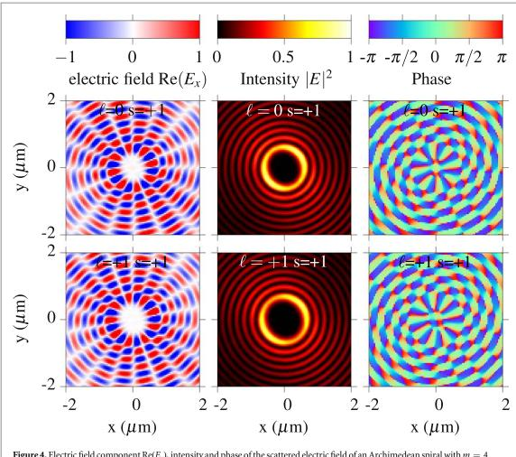
**Figure 4.** Electric field component  $\operatorname{Re}(E_{\chi})$ , intensity and phase of the scattered electric field of an Archimedean spiral with m = 4 elements for an excitation with OAM values of  $\ell = 0, +1$  and circular polarization s = +1 at the wavelength  $\lambda = d/2 = 400$  nm.
