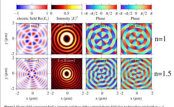
**Figure 2.** Electric field component  $\text{Re}(E_x)$ , intensity and phase of the scattered electric field of an Archimedean spiral with m = 4 elements for plane wave excitation with varying polarization  $s = \pm 1$ . The refractive index of the embedding medium is n = 1 (top row) and n = 1.5 nm (bottom row).
