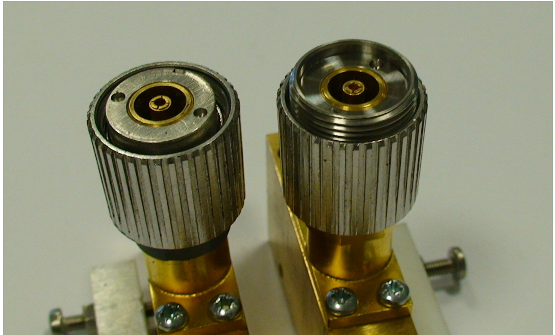
Fig A1.2.1 The APC-7 Connector showing the genderless contact faces, the threaded retaining rings screw back into each knurled nut, so a male or female thread can be set on any part.
