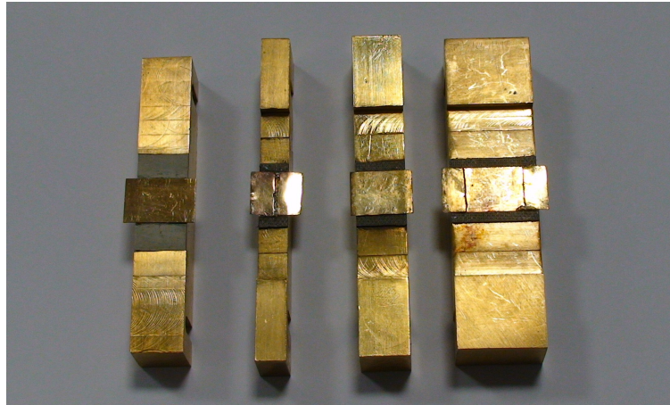
Fig A1.3.1 The 10 ohm line references, also shown left is a low impedance line.
