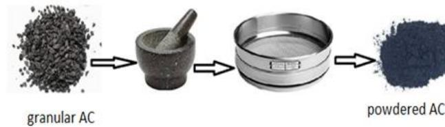
Figure 4-5 Grinding the granular activated carbon to powder
