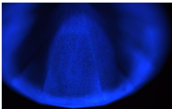
**Figure 3.** CMOS image showing the spatial distribution of the prompt blue luminescence signal exhibited by a typical type IIa natural diamond.
