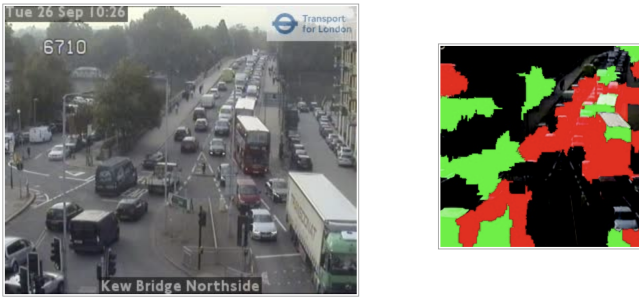
Figure 1: Example saliency map for traffic congestion: the red regions of the input image are most significant in classifying the image as congested
