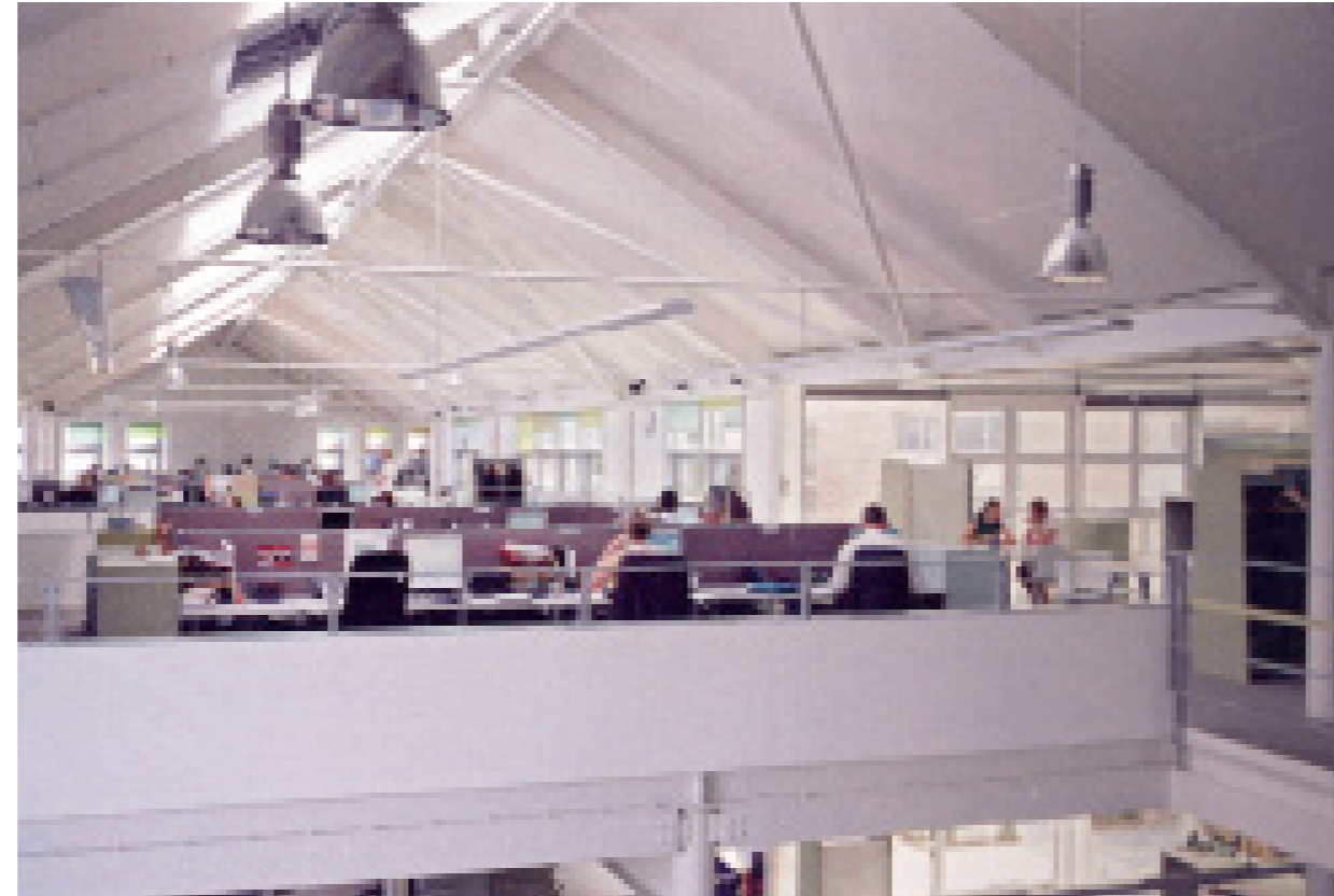
Over 100m long and 23m wide the building has the potential to accommodate a range of offices - in this form 2 bats of office share an atrium space to provide daylight and natural ventilation
