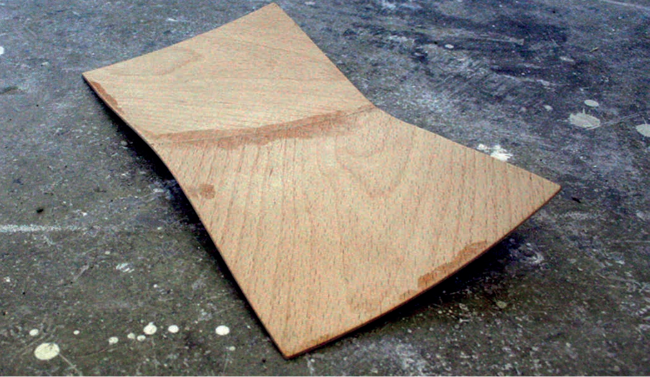
Figure 7: Haugen's Double Curved Plywood (from Michael Hensel & Sørensen, 2016 with the courtesy of Hensel)
