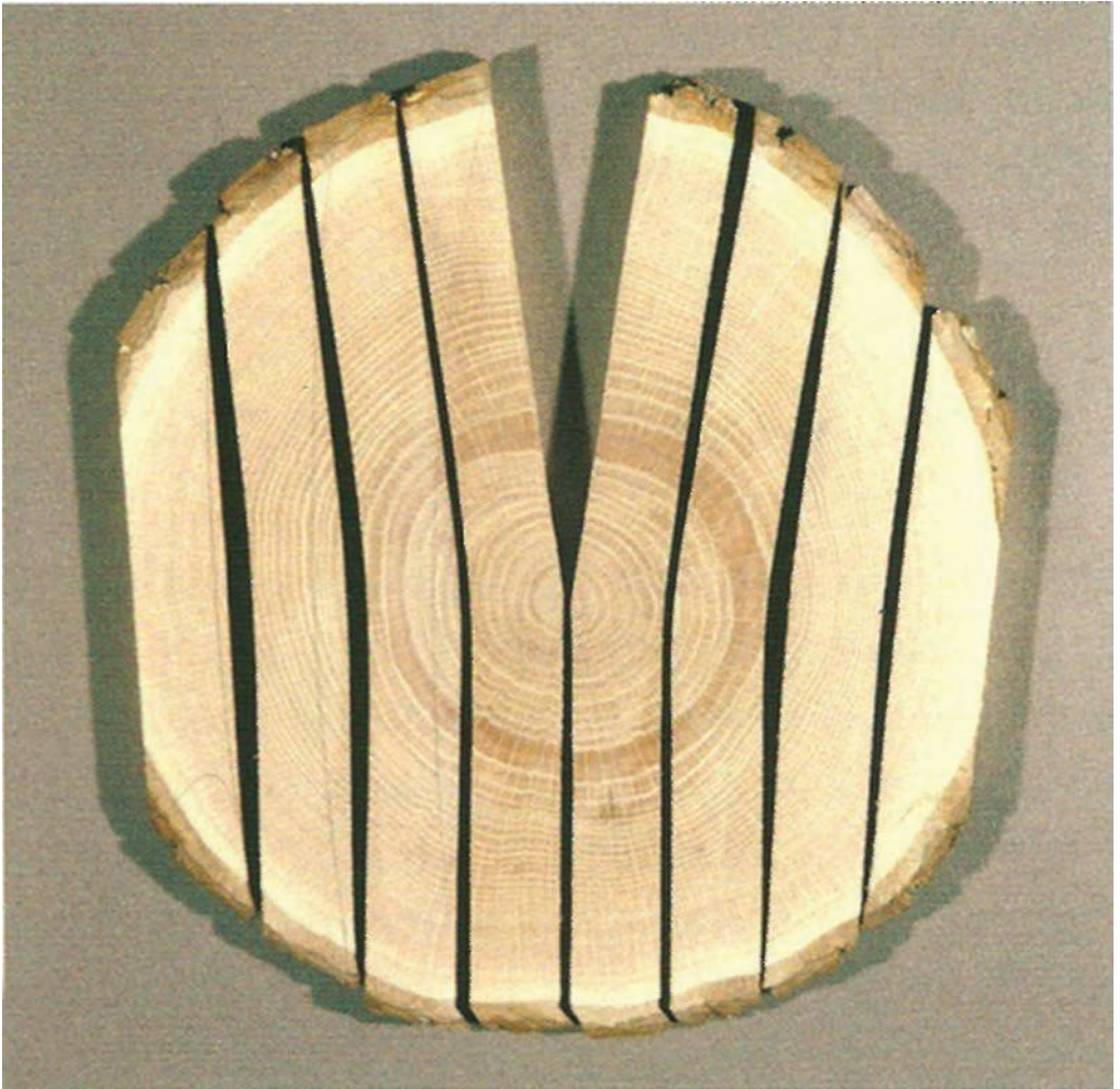
Figure 49: The severity of cupping in a board is related to its position in the log (photo: R. Bruce Hoadley from: Hoadley, 1980; with the courtesy of Taunton press)
