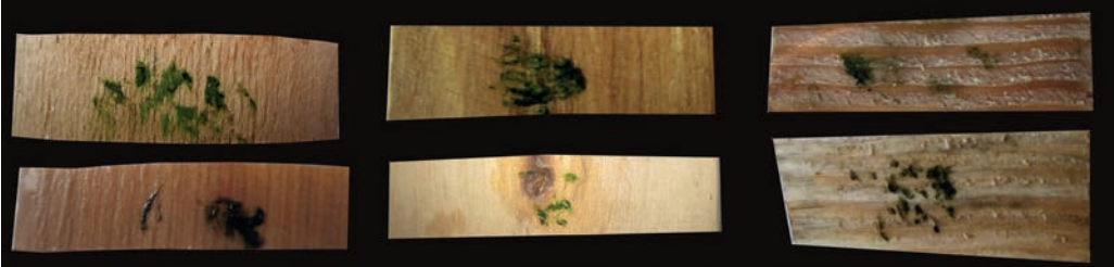
Figure 55: Samples of Artificial Growth of Apatococcus and Klebsormidium (from up to down) on Ash, False Acacia and Pine Wood from Left to Right, Respectively (Davidová 2013)
