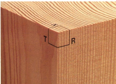
Figure 2: This block of Douglas-fir was cut to show three planes: the transverse or cross-sectional surface (X), the radial surface (R), and the tangential surface (T) (photo by Randy O'Rourke from Hoadley, 1980 with the courtesy of Taunton Press)
