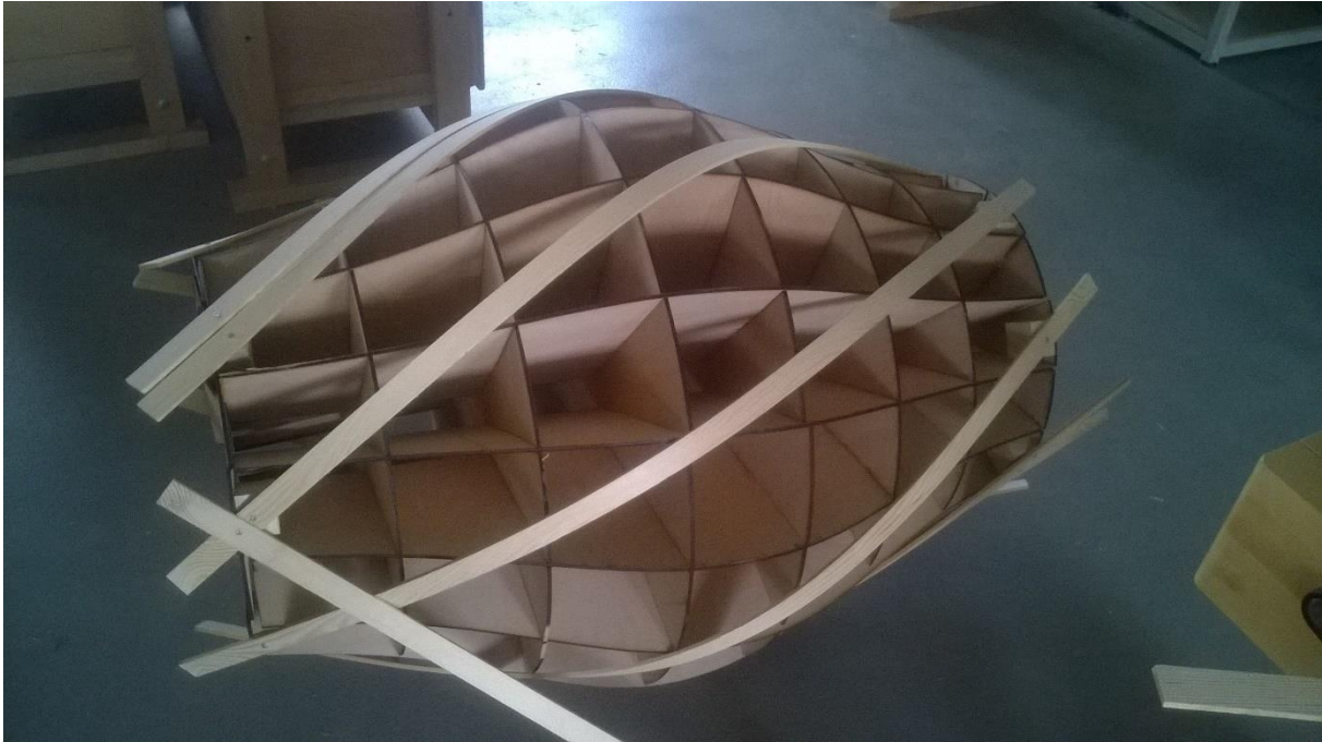
Figure 8: The Prototype Trial that Structurally Failed to Perform (Photo: Davidová 2017)
