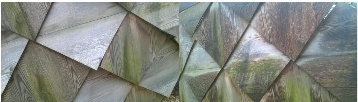
Figure 18: Ray 2 Responsive Wood Envelope Prototype a) in semi-dry April weather when the screen is partly open for boundary exchange between the exterior and semi interior; b) After April light rain when the System is closed, not allowing the humid and cold air to pass through the boundary; both after four years of exposure to weather and biotic conditions. The prototype became inhabited by Blue Stein Fungi, Algae and Lichen. These, especially the algae, regulate the moisture content of the wood, thus contributing to its warping. Notice also the organisation of Algae habitation caused by the material's fibre direction and position within the design that is affected by material performance and form. Thus, it is organised through its moisture and the organism's abundance and distribution interaction (Photo: Davidová 2017) (Davidová, 2017)
